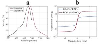
Fig. 6 PL spectra (a) of  $SiO_2$ -Lys-SP-NCs, with excitation (black) and emission (red) plots, highlighting excitation maximum at 675 nm and emission maximum at 690 nm. Magnetization curves (b) of  $SiO_2$ -Cit-SP-NCs (blue) and  $SiO_2$ -Lys-SP-NCs (red), normalized to the inorganic content.
