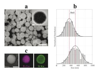
Fig. 5 SEM micrograph (a) of  $SiO_2$ -Lys-SP-NCs. Scale bar of 1  $\mu$ m. In the inset, TEM micrograph of a single-NC with a scale bar of 100 nm. Dry size distribution and Gaussian fit comparison (b) between uncoated (top,  $R^2 = 98\%$ ) and coated (bottom,  $R^2 = 88\%$ ) SP-NCs, highlighting the (double) shell thickness (170 nm). EDX mapping (c) of a single SiO<sub>2</sub>-Lys-SP-NC, detecting Fe Lα and Si Kα characteristic X-ray emission lines. Scale bar indicates 250 nm.
