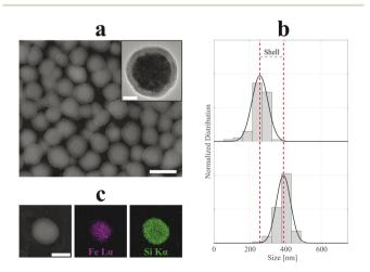
Fig. 4 SEM micrograph (a) of SiO<sub>2</sub>-Cit-SP-NCs. Scale bar of 500 nm. In the inset, TEM micrograph of a single-SP-NC with a scale bar of 50 nm. Dry size distribution and Gaussian fit comparison (b) between uncoated (top,  $R^2 = 95\%$ ) and coated (bottom,  $R^2 = 97\%$ ) SP-NCs, highlighting the (double) shell thickness (130 nm). EDX mapping (c) of a single SiO<sub>2</sub>-Cit-SP-NC, detecting Fe Lα and Si Kα characteristic X-ray emission lines. Scale bar indicates 250 nm.
