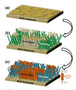
Fig. 4 Depicts a schematic representation of the GaN-based NW fabrication flow: (a) aggregation of the Au/Ga/In metal alloy catalyst, (b) formation of the GaN core NWs, and (c) InGaN/GaN MQW coaxial shells on the BeO substrate; the inset indicates the geometry of the core/shell structure. Reproduced with permission from ref. 81. Copyright 2020 ACS publisher.
