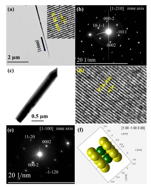
Fig. 14 (a) TEM image of pristine GaN NWs, in which inset shows magnified lattice fringes, (b) SAED pattern of pristine GaN NWs, (c) TEM image of coaxial GaN NW, (d) magnified fringes of a coaxial GaN NW, (e) SAED pattern of coaxial GaN NWs, and (f) model of wurtzite GaN crystal structure oriented along the *c*-axis. Reproduced with permission from ref. 87. Copyright 2021 Elsevier publisher.
