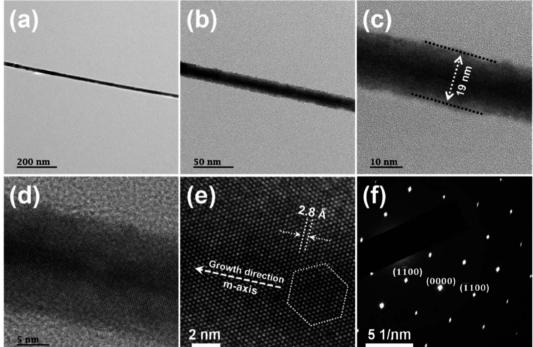
Fig. 6 Transmission electron micrographs of GaN core NWs grown on a BeO substrate: (a-c) low- to high-magnification images, (d) high-magnification image showing planes with the complete width, (e) interplanar spacing along the m-axis with a very clear growth direction, and (f) SAED patterns verifying the growth direction along the m-axis. Reproduced with permission from ref. 81. Copyright 2020 ACS publisher.
