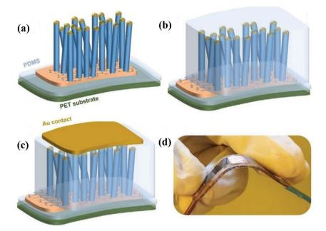
Fig. 15 (a) Transfer of GaN NWs grown on a graphene-coated Cu foil onto a PDMS-coated PET substrate. (b) PDMS deposition to build a GaN NW-PDMS matrix on the substrate. (c) Au evaporation onto the PENG. (d) Image of the full device's corresponding structure. Reproduced with permission from ref. 55. Copyright 2020 Wiley publisher.
