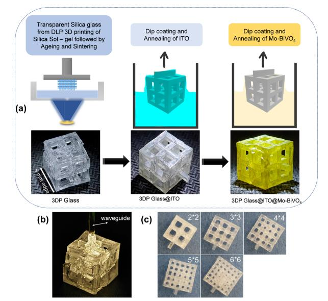
Fig. 1 (a) Illustration of the fabrication of semi-transparent 3D lattice structures for photoelectrochemical water oxidation. (b) Picture of the 3D printed glass in a dark room with a light waveguide joined at the tip of the lattice to demonstrate waveguiding of the light through the lattice structure. (c) Picture of the 3D printed glass lattice structures with varying degrees of porosity; all the printed lattices have the dimension of a 9 mm  $\times$  9 mm  $\times$  9 mm cube.
