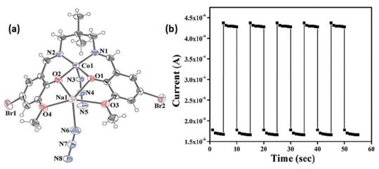
Fig. 4 (a) A thermal ellipsoid plot of a hetero-binuclear unit of 15 drawn with 40% ellipsoidal probability; (b) conductivity of the ITO/15/Al configuration under light-on and light-off conditions. Reproduced with permission from ref. 63. Copyright 2019 Royal Society of Chemistry.
