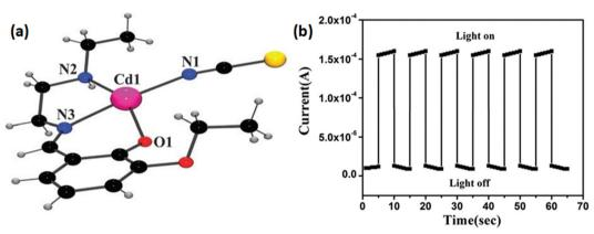
Fig. 2 (a) A perspective view of the asymmetric unit of 1; (b) conductivity of ITO/1/Al configuration at light-on and light-off conditions. Reproduced with permission from ref. 53. Copyright 2015 Royal Society of Chemistry.
