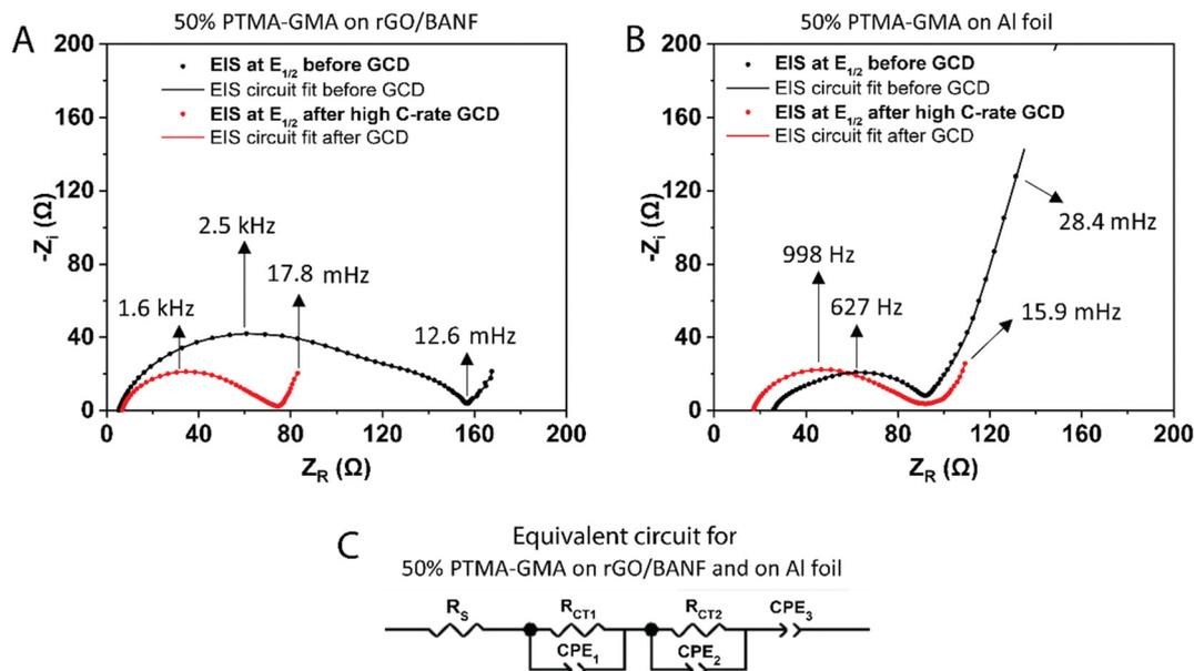
Fig. 5 EIS at the half-wave potential ( $E_{1/2} = 3.66$  V) for 50 wt% PTMA-GMA on (A) rGO/BANF and (B) Al foil before and after rate capability testing. (C) Fitted equivalent circuit for 50 wt% PTMA-GMA on rGO/BANF and Al foil.
