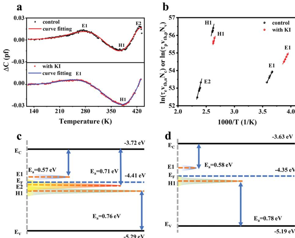
Fig. 8 (a) DLTS signals for the device without and with KI post-treatment. (b) Corresponding Arrhenius plots obtained from the DLTS signals. Position distribution of CBM ( $E_c$ ), VBM ( $E_v$ ), Fermi level ( $E_F$ ) and defect energy level for  $\text{Sb}_2(\text{S,Se})_3$  films (c) without and (d) with KI post-treatment. Adapted with permission from ref. 85 Copyright 2022, Wiley-VCH.
