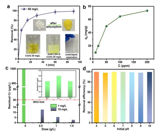
Fig. 4 (a) Sorption kinetics of  $Cr^{VI}$  by ZnAl-LDH-D (dose = 0.5 g  $L^{-1}$ ,  $C_0$  = 50 mg  $L^{-1}$ ); (b) sorption isotherms of  $Cr^{VI}$  by ZnAl-LDH-D (dose = 0.5 g  $L^{-1}$ ,  $C_0$  =10–200 mg  $L^{-1}$ , t = 2 h); (c) deep adsorption performance of ZnAl-LDH-D toward  $Cr^{VI}$  with a low concentration (t = 2 h); (d) influence of the initial pH on the adsorption performance (dose = 0.5 g  $L^{-1}$ ,  $C_0$  = 50 mg  $L^{-1}$ , t = 2 h).
