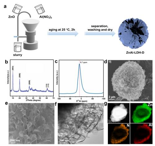
Fig. 1 (a) Schematic illustration for the production of ZnAl-LDH-D; (b) XRD pattern of ZnAl-LDH-D; (c) <sup>27</sup>Al MAS NMR spectrum of ZnAl-LDH-D; (d) and (e) SEM images of ZnAl-LDH-D; (f) and (g) TEM image and corresponding EDX mappings of ZnAl-LDH-D.
