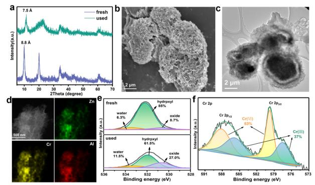
Fig. 5 (a) XRD patterns of ZnAl-LDH-D before and after adsorption of Cr<sup>VI</sup>; (b) SEM image of ZnAl-LDH-D after adsorption of Cr<sup>VI</sup>; (c) and (d) TEM image and the EDS mapping of ZnAl-LDH-D after adsorption of Cr<sup>VI</sup>; (e) high-resolution XPS O 1s spectra of ZnAl-LDH-D before and after adsorption of Cr<sup>VI</sup>; (f) high-resolution XPS Cr 2p spectra of ZnAl-LDH-D after adsorption of CrVI
