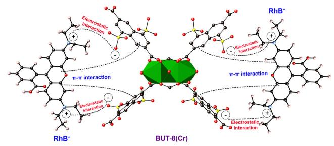
Scheme 1 The plausible adsorption mechanism of RhB+ onto BUT-8(Cr). Atom colors: Cr, green polyhedra; C, black; O, red; S, yellow; N, blue.
