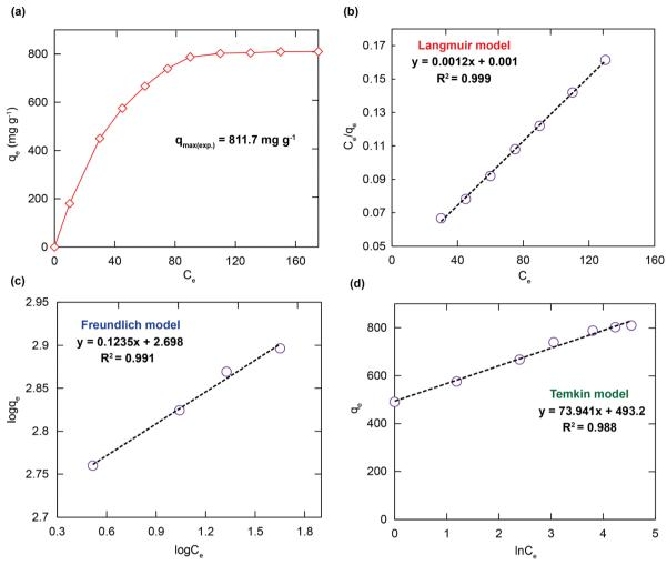
Fig. 5 Effect of the concentration of RhB on the adsorption capacity of H<sup>+</sup> $\subset$ BUT-8(Cr) [m = 10 mg,  $V_{RhB} = 100 \text{ mL}$ ,  $C_0$ : 25–175 mg L<sup>-1</sup>, pH = 3, t = 24 hJ(a); fitting results with the adsorption isotherm models: Langmuir (b), Freundlich (c), and Temkin (d)
