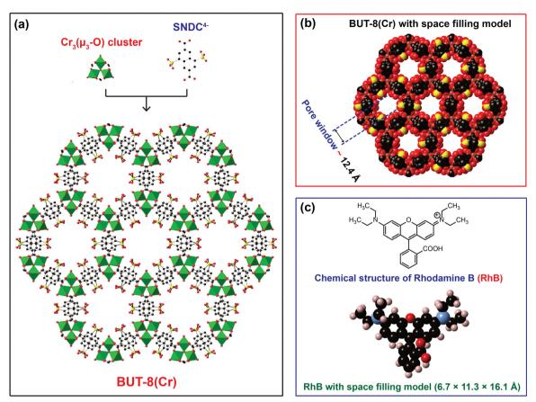
Fig. 1 The structure of  $H^+ \subset BUT-8(Cr)$  constructed from the  $Cr_3(\mu_3-O)$  clusters and  $SNDC^{4-}$  linker (a); the pore window of BUT-8(Cr) with the space filling model (b); the chemical structure and space filling model of RhB (c). Atom colors: Cr, green polyhedra; C, black; O, red; S, yellow; N, blue. Almost H atoms are omitted for clarity.
