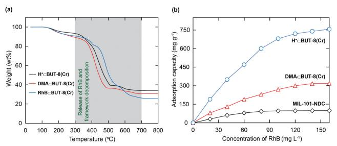
Fig. 3 (a) TGA curves of activated  $H^+ \subset BUT - 8(Cr)$  (black), activated DMA $\subset BUT - 8(Cr)$  (red), and activated RhB $\subset BUT - 8(Cr)$  (blue); (b) dependence of the sulfonic groups within the structures of MIL-101-NDC, DMA $\subset BUT - 8(Cr)$  and  $H^+ \subset BUT - 8(Cr)$  on the RhB adsorption capacity.
