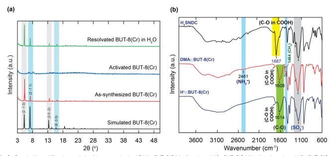
Fig. 2 Powder X-ray diffraction analysis of the as-synthesized DMA $\subset$ BUT-8(Cr) (red), activated H $^+$  $\subset$ BUT-8(Cr) (blue), and resolvated H $^+$  $\subset$ BUT-8(Cr) in water (green) in comparison with simulated BUT-8(Cr) (black) (a); Fourier transform infrared spectra of the  $H_4$ SNDC linker (black), DMA  $\subset$  BUT-8(Cr) (red), and  $H^+ \subset BUT-8(Cr)$  (blue) (b).
