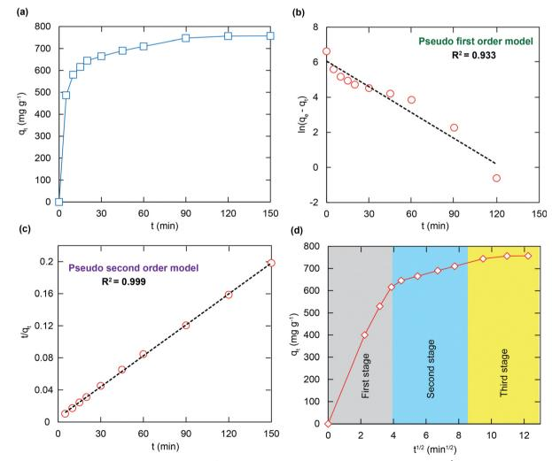
Fig. 6 The kinetic curve for the adsorption of RhB onto H<sup>+</sup>  $\subset$  BUT-8(Cr) [m = 10 mg,  $V_{RhB} = 100$  mL,  $C_0 = 100$  mg L<sup>-1</sup>, pH = 3] (a); data fitting with the adsorption kinectic models: pseudo first order (b), pseudo second order (c) and intra-particle diffusion model (d)
