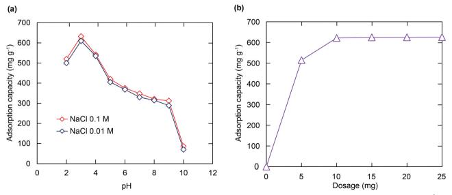
Fig. 4 Influence of solution pH value and ionic strength on the adsorption capacity of RhB over H<sup>+</sup> $\subset$  BUT-8(Cr) [m = 10 mg,  $C_0 = 200$  mg L<sup>-1</sup>,  $V_{RhB} = 10$ 50 mL, t = 24 h] (a); Effect of H<sup>+</sup>  $\subset$  BUT-8(Cr) content on the RhB adsorption uptake [m: 5–25 mg,  $C_o = 200$  mg L<sup>-1</sup>,  $V_{RhB} = 100$  mL, pH = 3, t = 24 h] (b).
