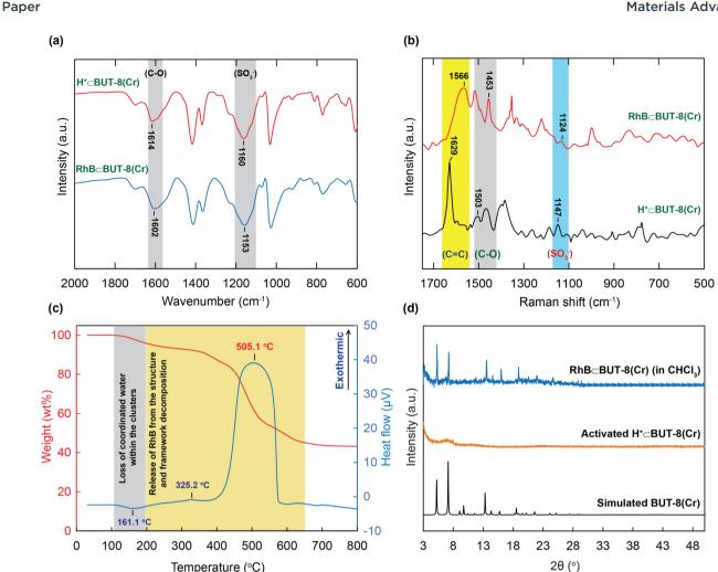
Fig. 8 Fourier transform infrared spectra of RhB⊂BUT-8(Cr) (blue) as compared to those of H<sup>+</sup>⊂BUT-8(Cr) (red) (a); Raman spectra of RhB⊂BUT-8(Cr) (red) in comparison with those of H+ BUT-8(Cr) (black) (b); TGA diagram (red) and DSC curve (blue) of activated RhB BUT-8(Cr) (c); powder X-ray diffraction analysis of RhB = BUT-8(Cr) (RhB solution with CHCl<sub>3</sub>) (blue), activated H<sup>+</sup> = BUT-8(Cr) (orange) in comparison with simulated BUT-8(Cr) (black) (d)
