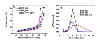
Fig. 9 (A) N<sub>2</sub> adsorption-desorption isotherms, and (B) pore radius distributions of ZNTC\_600, ZNTP\_600, and ZNTC\_600\_CNC
