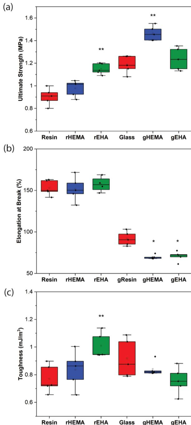
Fig. 4 (a) Ultimate strength, (b) elongation at break, and (c) toughness for neat and glass microsphere-filled samples. Individual data points as well as box and whisker plots are presented. \* indicates statistical differences from the control (either Resin or gResin). \*\* indicates statistical differences from all other conditions of the same type of sample (either neat or glass microsphere-filled).
