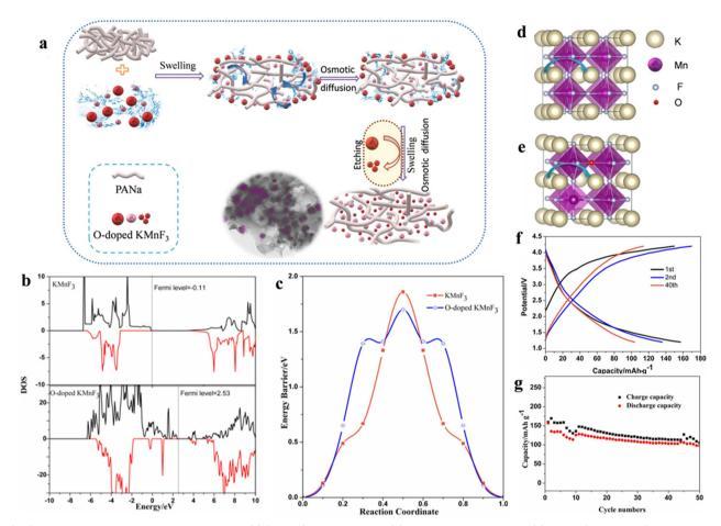
Fig. 9 Schematic diagram of the synthesis process. (a) Charge/discharge curves (b) and cycling performance (c) of KMnO<sub>0.125</sub>F<sub>2.875</sub>. Spin polarization of DOS (d) and energy profile (e). Schematic diagram of K migration (f and g). 110 Copyright © 2020 Elsevier.
