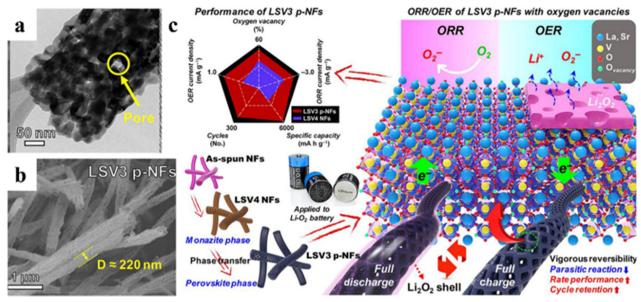
Fig. 13 TEM (a) and SEM (b) of La<sub>0.8</sub>Sr<sub>0.2</sub>VO<sub>3</sub> (LSV3 p-NFs). Schematic illustration of LSV3 p-NFs used in rechargeable Li-O<sub>2</sub> batteries (c). Temperature (c) and SEM (b) of La<sub>0.8</sub>Sr<sub>0.2</sub>VO<sub>3</sub> (LSV3 p-NFs). Schematic illustration of LSV3 p-NFs used in rechargeable Li-O<sub>2</sub> batteries (c). 2020 Elsevier.
