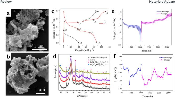
Fig. 11 SEM of LaNi<sub>x</sub>Mn<sub>1-x</sub>O<sub>3</sub> (x = 0.2) (a) and LaMnO<sub>3</sub> (b). Charge/discharge curves (c), XRD at different voltages (d), GITT curves (e) and diffusion coefficients (f) of LaNi<sub>x</sub>Mn<sub>1-x</sub>O<sub>3</sub> (x = 0.2). Copyright © 2022 Elsevier.
