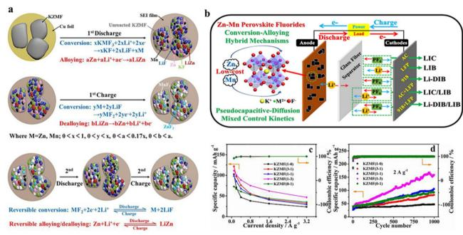
Fig. 5 Reaction mechanism of the KZMF electrode (a). Schematic diagram of potential applications of KZMF for Li<sup>+</sup> storage (b). Specific capacity of KZMF (c) and cycling performance (d). 70 Copyright © 2020 Elsevier.
