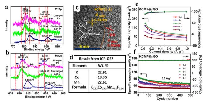
Fig. 8 Co2p (a) and Mn2p (b) of KCMF(1-1)@rGO at different voltage points (ex situ XPS). TEM (c) and ICP-OES (d) of KCMF(1-1)@rGO samples. The capacity and coulombic efficiency of KCMF@rGO with different Co/Mn ratios were obtained in the fifth cycle (e). Cycling stability (f). 101 Copyright © 2021 Elsevier.
