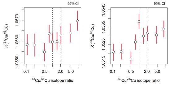
Fig. 1 The estimates of instrumental isotope ratio correction factors ( $K_{63/65}$ ) from two measurement sequences (set 1) depending on the isotope ratio of copper ( $r_{63/65}$ ) in the gravimetric mixtures of materials A and B (Table 1). Two dotted vertical lines correspond to  $r_{63/65} = 1:1$  (best measurements) and  $r_{63/65} = 2.24$  (natural copper).
