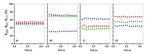
Fig. 8 Conversion of pure DEE ( $X_{\text{DEE}}$ , red) and selectivity of ethylene ( $S_{\text{ETY}}$ , green) and of ethanol ( $S_{\text{ET}}$ , blue) as a function of TOS for: (A) HZ(23), (B)  $HZ(23)_0.1OH$ , (C) HZ(80), and (D)  $HZ(80)_1.0OH$  catalysts. Test conditions: 225 °C, 1 bar and WHSV = 35.7 h<sup>-1</sup>.
