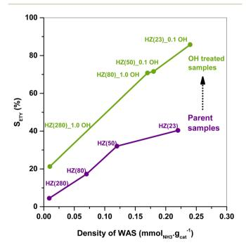
Fig. 2 Correlation between the ETY selectivity (at similar ET conversion) and the density of WAS for parent (purple) and OH-treated (green) HZSM-5 catalysts tested at 225 °C, 1 bar, WHSV = 35.7 h<sup>-1</sup>. S<sub>ETY</sub> data are obtained under stable catalytic behaviors.
