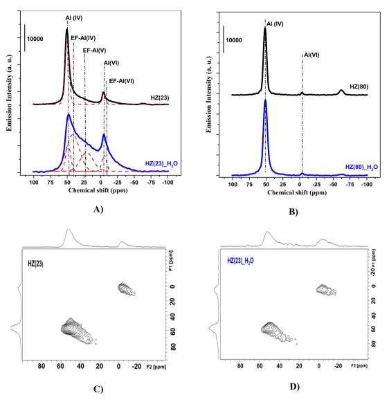
Fig. 4 27Al MAS-NMR spectra of (A) parent HZ(23) and water-treated HZ(23); (B) HZ(80) and water-treated HZ(80). The (C) and (D) figures represent <sup>27</sup>Al 3QMAS-NMR data for HZ(23) and HZ(23)\_H<sub>2</sub>O respectively.
