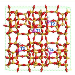
**Fig. 9** The optimized periodic structure of HZSM-5 (atomic ratio Si/Al  $\sim$ 23, a=20.615223 Å; b=20.430119 Å and c=13.716548 Å,  $\alpha=90.0248$ ;  $\beta=89.76483$ ;  $\gamma=90.05055$ ). Yellow: Si; red: O; purple: Al; white: protons.
