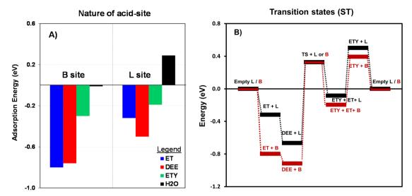
Fig. 10 (A) The calculated adsorption energy (eV, eqn (8)) for ET, DEE, ETY and H<sub>2</sub>O on B sites and L sites for the T2 position (-Al-); and (B) Reaction coordinate diagram with DFT-derived energies normalized with respect to empty B or L sites at T2 positions. The TS for ET → DEE is not shown for simplicity.
