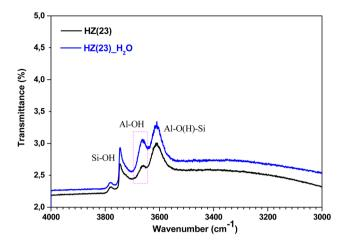
Fig. 5 Normalized FTIR spectra of the OH-region for fresh parent HZ (23) and HZ(23)\_H<sub>2</sub>O samples evacuated *in situ* at 350 °C (overnight) after  $ex\ situ$  calcination at 500 °C (5 h).
