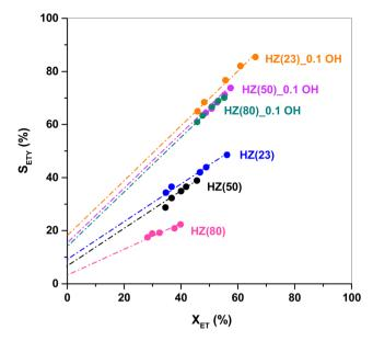
Fig. 7 ETY selectivity ( $S_{\text{ETY}}$ ) as a function of ET conversion ( $X_{\text{ET}}$ , changed with WHSV) over HZ(23), HZ(50), HZ(80), HZ(23)\_0.1 OH, HZ (50)\_0.1 OH and HZ(80)\_0.1 OH. Test conditions: 225 °C, total pressure  $\sim$ 1 bar. WHSV = 17.9-89.1 h<sup>-1</sup>.
