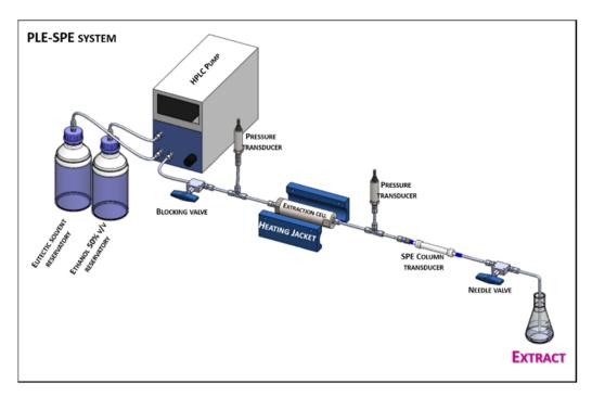
Fig. 1 Simplified diagram of the PLE-SPE system used (see the complete diagram of the equipment used in Viganó et al. (2021).<sup>17</sup>
