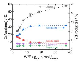
Fig. 3 Acetone conversion and product yields as a function of contact time for Siralox 30 at 260 °C. The dotted lines are only for visual quidance.
