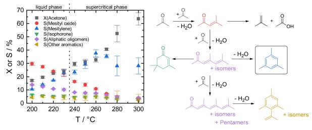
Fig. 2 Left: acetone conversion and product selectivity for Siralox 30 at different reaction temperatures (WHSV = 7.8 h<sup>-1</sup>, 75 bar) in liquid and supercritical acetone. Error bars give the standard deviation of the GC measurements at steady-state conditions. Right: a simplified network of the acid-catalyzed self-condensation of acetone.
