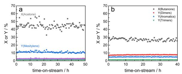
Fig. 4 Stability test of Siralox 30 under optimized reaction conditions (260 °C, 12.5  $g_{cat}$  h mol<sup>-1</sup>, WHSV = 4.7 h<sup>-1</sup>) in the conversion of acetone (a) and 2-butanone (b). Other products depicted in 4a:  $\bullet$  Y(Mesityl oxide),  $\nabla$  Y(Isophorone),  $\diamond$  Y(Oligomers).
