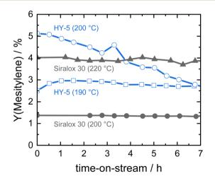
Fig. 1 Catalyst stability of silica-alumina HY-5 and Siralox 30 based on mesitylene yield at different reaction temperatures (7.8  $h^{-1}$ , 40 bar).
