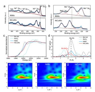
Fig. 3 XPS and XAS spectral characterization. (a) Ni 2p and (b) Mo 3d XPS spectra. (c) Mo K-edge XAS and (d) the corresponding  $k^2$ -weighted FT of EXAFS spectra in R space. (e)–(g) Wavelet transforms for the  $k^3$ -weighted EXAFS signals at the Mo K-edge of Mo foil, NiMo and NiCuMo, respectively.
