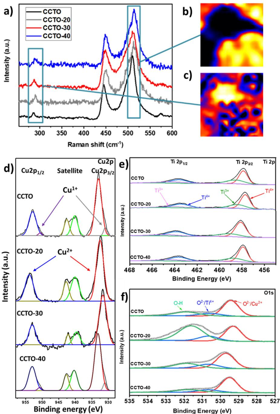
Fig. 4 (a) Raman shifts of the CCTO samples prepared using different PMMA amounts (0, 20, 30, and 40 wt%). (b and c) Raman maps: (b) 510  $\text{cm}^{-1}$  (CCTO) and (c) 291  $\text{cm}^{-1}$  (CuO). (d–f) High-resolution XPS spectra of (d) Cu 2p<sub>3/2</sub>, (e) Ti 2p<sub>3/2</sub>, and (f) O 1s for the CCTO samples prepared using different PMMA amounts (0, 20, 30, and 40 wt%).
