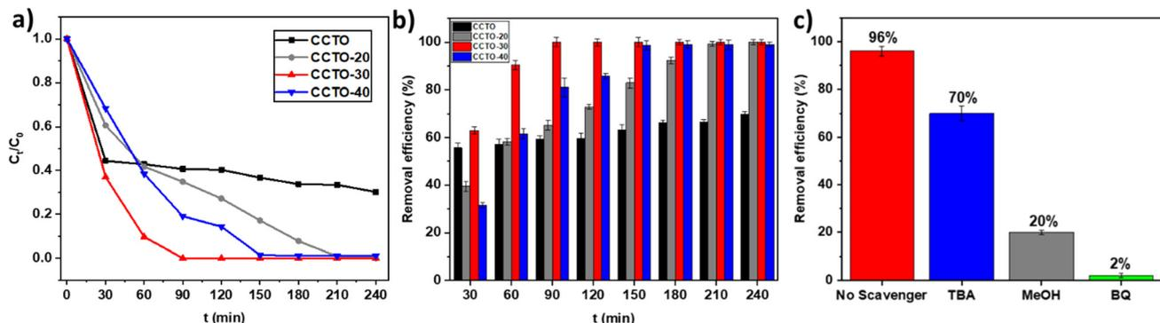
Fig. 7 (a) PCM degradation by electrocatalysis via PMS activation. (b) PCM removal efficiency. (c) Radical scavengers test. TBA: *tert*-butanol ( $\cdot\text{OH}$  scavenger); MeOH: methanol ( $\cdot\text{OH}$  and  $\cdot\text{SO}_4^-$  scavenger); BQ: *p*-benzoquinone ( $\cdot\text{O}_2^-$  scavenger).
