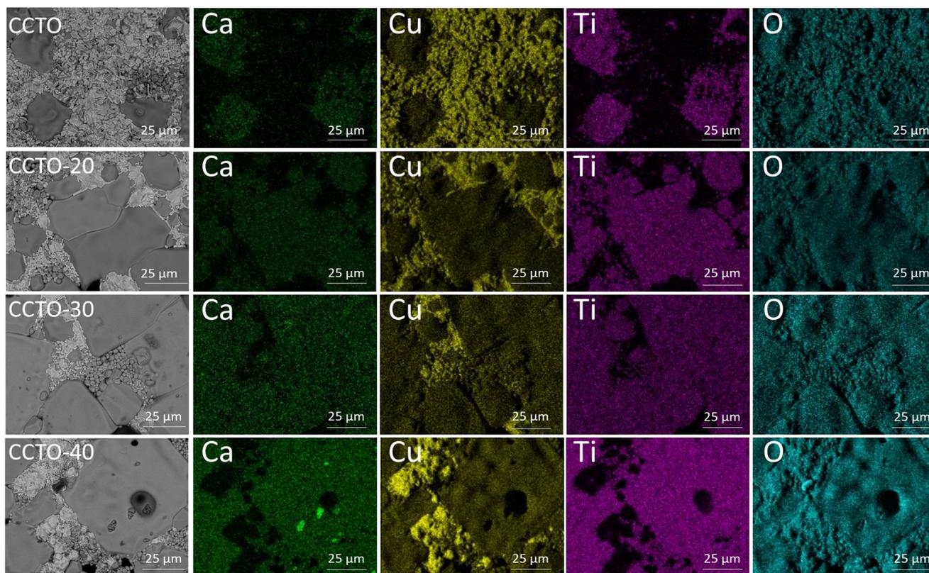
**Fig. 2** SEM/EDX mapping of the CCTO samples prepared using different PMMA amounts (0, 20, 30, and 40 wt%).
