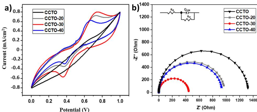
Fig. 6 (a) Cyclic voltammograms obtained using CCTO, CCTO-20, CCTO-30 and CCTO-40 as electrodes in 1 M KOH (scan rate = 25 mV s<sup>-1</sup>). (b) Nyquist plots showing the electrochemical impedance spectroscopy data for CCTO, CCTO-20, CCTO-30 and CCTO-40.
