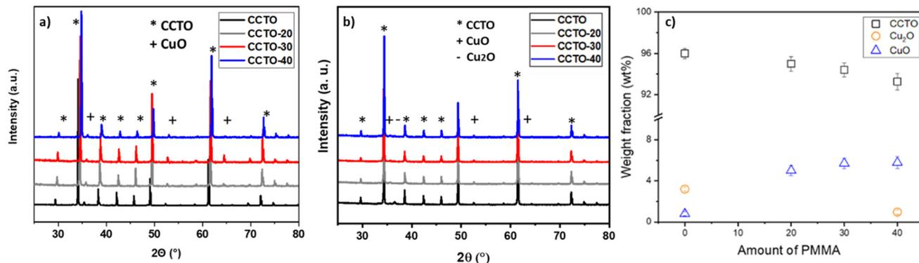
**Fig. 3** (a) XRD patterns of CCTO pellets prepared using different amounts of PMMA (0, 20, 30, and 40 wt%). (b) XRD patterns of the same samples after powdering. (c) Weight fraction of the formed crystalline phases (Rietveld analysis of the XRD data for the powdered samples).
