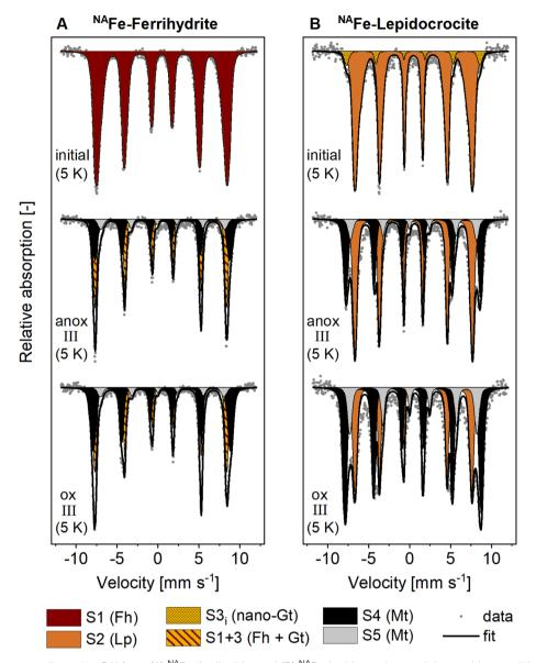
Fig. 3 Mössbauer spectra collected at 5 K from (A)  $^{NA}$ Fe-ferrihydrite and (B)  $^{NA}$ Fe-lepidocrocite mesh bags without soil before the incubation (initial) and after the incubation in the redox fluctuating mesocosms (redox cycle III anoxic and oxic period). Averaged fitting parameters and interpretations of Mössbauer fit components are given in Table 1, all fitting parameters are presented in Tables S11 and S12.† Abbreviations: anox = anoxic, ox = oxic, S = S
