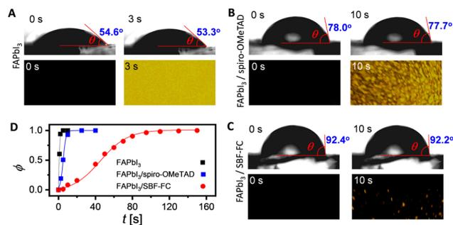
**Fig. 5** (A–C) Temporal evolutions of the water contact angle ( $\theta$ ) and the polarized optical microscopy (POM) image upon dripping a water droplet on three samples: (A) FAPbI<sub>3</sub>, (B) spiro-OMeTAD covered FAPbI<sub>3</sub>, and (C) SBF-FC covered FAPbI<sub>3</sub>. The size of the POM image is 500  $\mu$ m  $\times$  250  $\mu$ m. In the yellow region, perovskite is decomposed. (D) Plots of the yellow region percentage ( $\phi$ ) as a function of time ( $t$ ).
