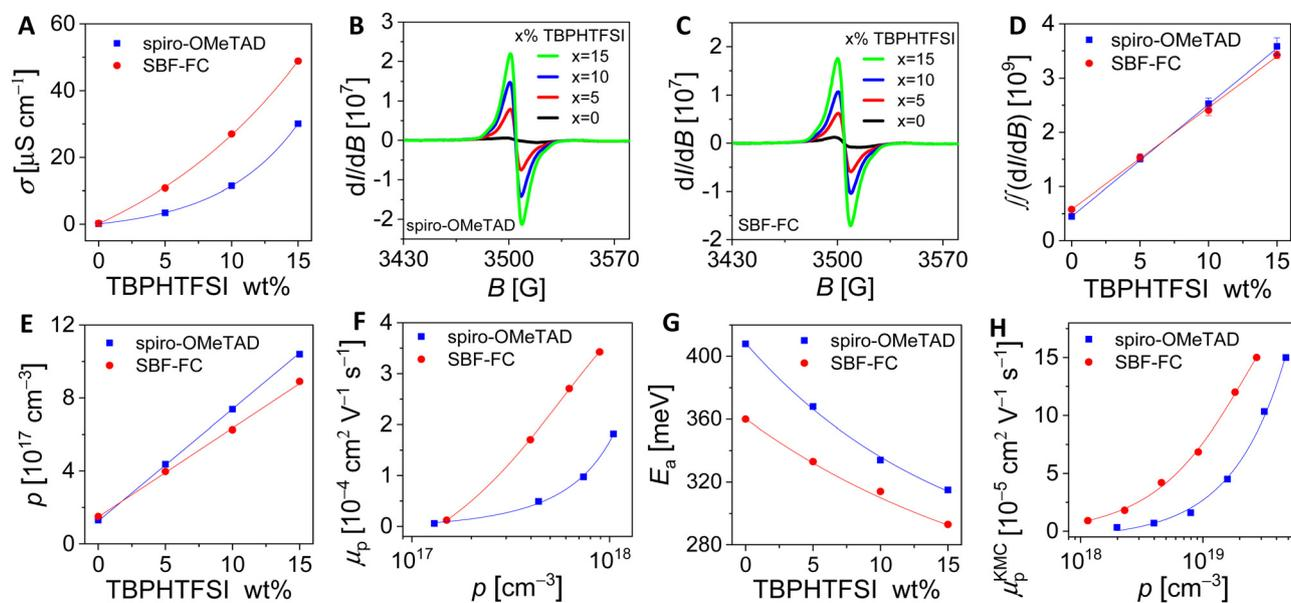
Fig. 2 (A) Plots of electrical conductivity ( $\sigma$ ) versus weight percentage (wt%) of TBPHTFSI. (B and C) Electron paramagnetic resonance spectra. Magnetic field strength,  $B$ ; first derivative of absorption intensity,  $dI/dB$ . (D) Quadratic integral of  $dI/dB$ . (E) Hole density ( $p$ ). (F) Plots of hole mobility ( $\mu_p$ ) versus  $p$ . (G) Activation energy ( $E_a$ ). (H) Kinetic Monte Carlo simulated hole mobility ( $\mu_p^{\text{KMC}}$ ).
