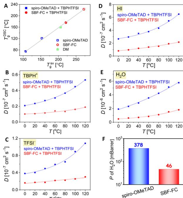
Fig. 4 (A) Correlation between theoretical and experimental glass transition temperatures. (B–E) Plots of the diffusion coefficient ( $D$ ) of species in the 15 wt% TBPHTFSI containing composites as a function of temperature ( $T$ ): (B) TBPH<sup>+</sup>; (C) TFSI<sup>-</sup>; (D) HI; and (E) H<sub>2</sub>O. (F) Theoretical permeability ( $P$ ) of H<sub>2</sub>O in the composites at room temperature.
