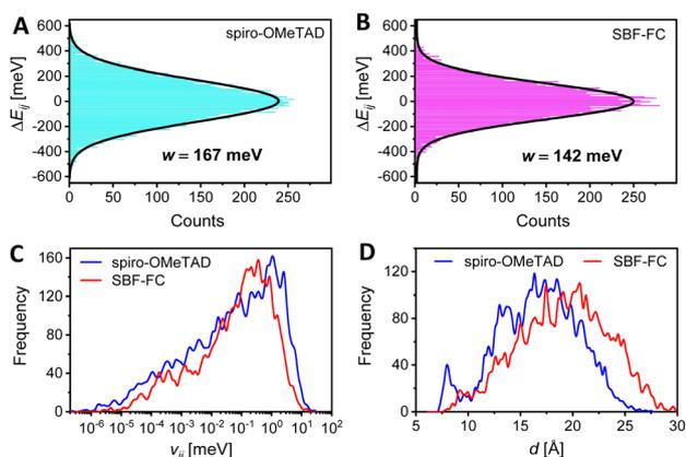
Fig. 3 (A and B) Distribution profiles of the HOMO energy level difference ( $\Delta E_{ij}$ ). The black solid lines refer to the Gaussian fits to acquire the energetic disorders, being 167 meV for spiro-OMeTAD and 142 meV for SBF-FC. (C and D) Profile of transfer integral ( $v_{ij}$ ) and centroid distance ( $d$ ).
