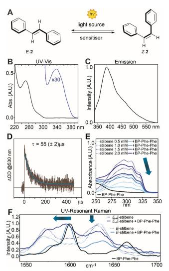
Fig. 3 (A) Photoisomerisation of E-stilbene (E-2). (B) UV-Vis spectra of BP-Phe-Phe. (C) BP-Phe-Phe emission spectrum (ex. 315 nm). (D) BP-Phe-Phe triplet state lifetime. (E) UV-Vis spectra of stilbene without and with BP-Phe-Phe (1 mM, cac). (F) UVRR spectra of BP-Phe-Phe, stilbene, and their mixtures, all in MeCN.
