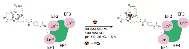
Fig. 3 Schematic description of no carrier-added radiochemical labeling procedure for the introduction of 89 Zr to the exogenous, DFO metal ion binding site of DFO-LanM.
