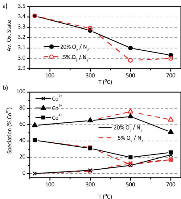
Fig. 8 Analysis of cobalt's oxidation state in LSC nanopowders as function of temperature and under different O<sub>2</sub> concentration in the O<sub>2</sub>/N<sub>2</sub> atmosphere. (a) Average oxidation state, and (b) speciation of cobalt atoms in LSC according to Co-K edge XANES analysis using the LCF method.
