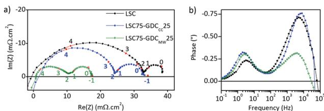
Fig. 4 (a) Nyquist plot of normalized EIS spectra and (b) bode-phase plot for LSC, LSC75–GDC<sub>CC</sub>25 and LSC75–GD<sub>MW</sub>25 cathodes at 700 °C under synthetic air flow. Inserted numbers close to red data points are their log(frequency) value. In (a), the pure resistive contribution of the electrolyte was subtracted from the data for easy comparison.
