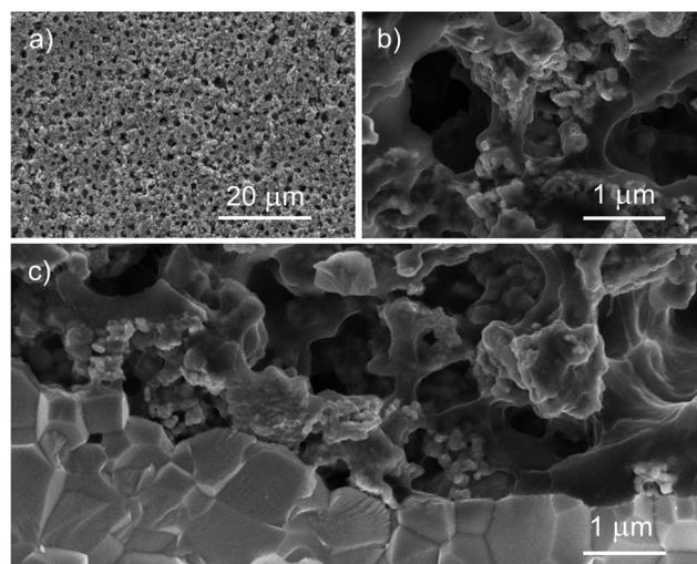
Fig. 1 SEM micrographs of LSC75–GDC<sub>CC</sub>25 cathode. (a) Top view at low magnification. (b) Detail of top view. (c) Cross section with SDC electrolyte at the bottom. The smallest particles in the cathode belong to the GDC phase.
