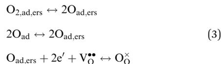
Eqn (3) shows that the process can consist of three steps: (1) dissociation of adsorbed  $O_2$ ; (2) diffusion of O atoms to *ers*; and (3) CT process. The analysis suggests that the CT process is present in both HF and MF arcs. This is possible because the HF arc is related to Langmuir's type oxygen absorption and the MF arc to oxygen adsorption with diffusion steps, and each process exhibits a different characteristic time.
