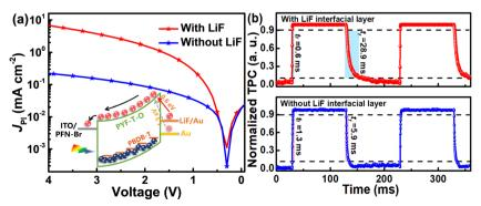
Fig. 3 PM-APDs with or without LiF layer: (a)  $J_{\rm Pl}-V$  curves, the inset depicts the effect of electron injection barrier on electron tunneling-injection. (b) Normalized TPC obtained at 850 nm light-illumination with the intensity of 1 mW cm<sup>-2</sup> under 4 V applied bias.
