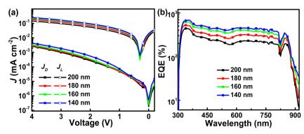
Fig. 2 (a) J-V curves and (b) EQE spectra under 4 V applied bias of PM-APDs.
