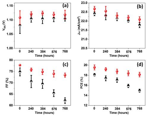
Fig. 5 The photovoltaic parameters ( $V_{OC}$ ,  $J_{SC}$ , FF and PCE) of the pristine (black colour) and 5 mg mL<sup>-1</sup> CBSC passivated perovskite solar cells (red colour) for the duration of 768 hours in the dried box.
