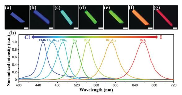
Fig. 2 The optical images of an isolated (a) ZJU-28  $\supset$  CsPbCl<sub>2</sub>Br, (b) ZJU-28  $\supset$  CsPbCl<sub>1.5</sub>Br<sub>1.5</sub>, (c) ZJU-28  $\supset$  CsPbClBr<sub>2</sub>, (d) ZJU-28  $\supset$  CsPbBr<sub>3</sub>, (e) ZJU-28⊃CsPbBr<sub>2</sub>I, (f) ZJU-28⊃CsPbBr<sub>15</sub>I<sub>1.5</sub> and (g) ZJU-28⊃CsPbBrl<sub>2</sub> microcrystals under excitation of 365 nm (for a-d) or 480 nm (for e-g). Scale bar, 50 μm. (h) PL spectra of the ZJU-28 ⊃ CsPbX<sub>3</sub> crystals.
