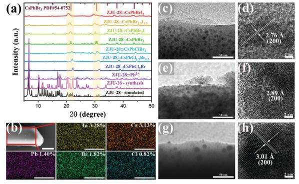
Fig. 1 (a) PXRD patterns of ZJU-28  $\supset$  Pb<sup>2+</sup> and ZJU-28  $\supset$  CsPbX3 crystals. (b) The SEM image of ZJU-28  $\supset$  CsPbClBr2 and the corresponding elemental mapping diagrams of In, Cs, Pb, Cl, and Br. Scale bar, 5  $\mu$ m. TEM image and HR-TEM image of (c and d) ZJU-28  $\supset$  CsPbBClBr2, (e and f) ZJU-28  $\supset$  CsPbBr3 and (g and h) ZJU-28  $\supset$  CsPbBr12.
