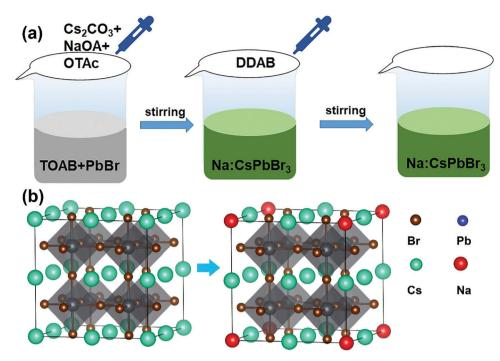
Fig. 1 (a) A schematic illustration of the synthesis procedure of Na<sup>+</sup>-doped CsPbBr<sub>3</sub> QDs. (b) A representative model of Na<sup>+</sup>-doped CsPbBr<sub>3</sub> QDs showing the replacement of some Cs positions with Na atoms
