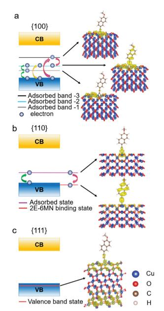
Fig. 9 Schematic illustration of the band diagrams and partial charge density distributions in real space for functionalized  $Cu_2O$  (a) {100}, (b) {110}, and (c) {111} surfaces.
