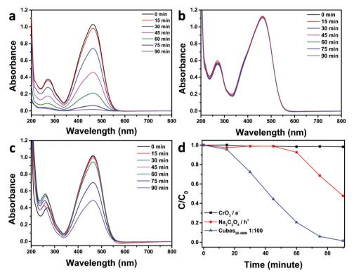
Fig. 5 UV-vis absorption spectra of methyl orange as a function of irradiation time using (a) 1:100 2E-6MN-modified  $Cu_2O$  cubes as the photocatalyst and in the presence of (b) 3  $\mu$ mol of  $CrO_3$  and (c) 3  $\mu$ mol of  $Na_2C_2O_4$ . (d) Summary of the electron and hole scavenger tests.
