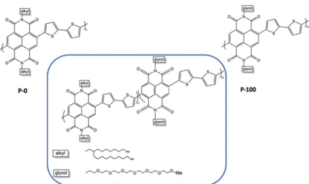
Fig. 10 Chemical structures of the investigated mixed conducting copolymers, the PO to P100 series. 37
