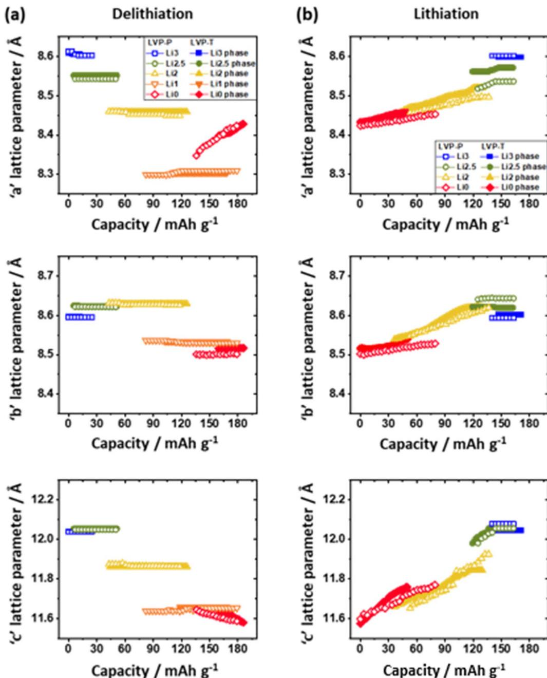
Fig. 5 Change in unit cell lattice parameters obtained from *in situ* XRD patterns of LVP-P (unfilled; reproduced from ref. 44 with permission from The Royal Society of Chemistry) and LVP-T (filled); "a," "b," and "c" lattice parameter in (a) the 1st charging (delithiation) and (b) discharging (lithiation) processes.
