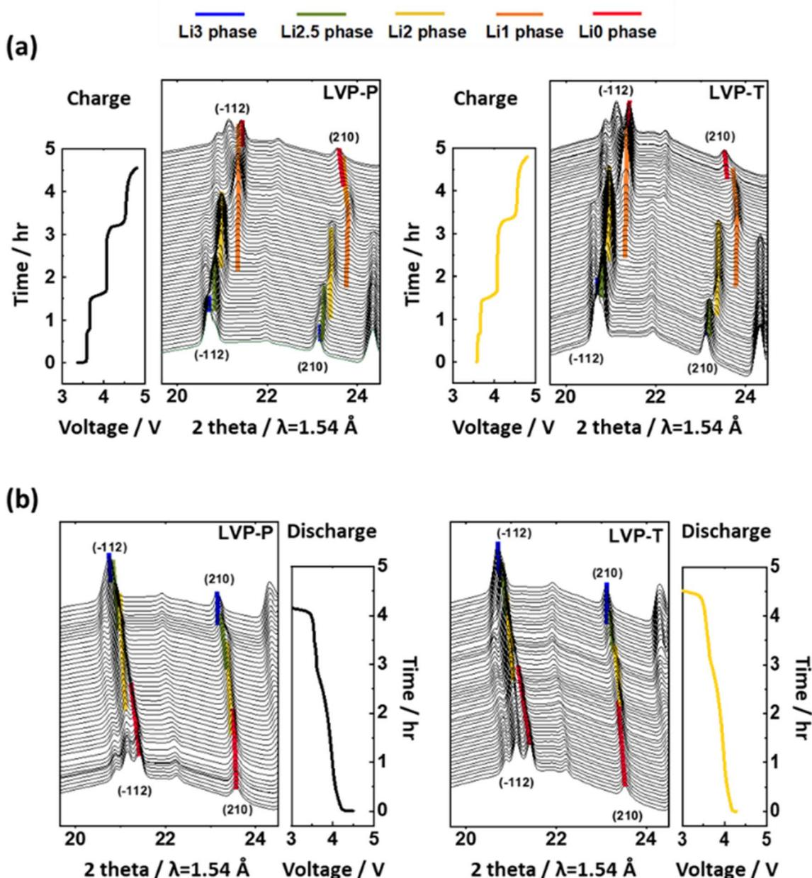
Fig. 4 *In situ* XRD patterns with time–voltage curve measured at 0.2C during the (a) 1st charge and (b) discharging process in the (–112), (210) planes of LVP-P (reproduced from ref. 44 with permission from The Royal Society of Chemistry) and LVP-T.
