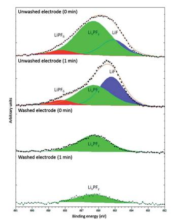
Fig. 6 F 1s XPS spectra (Al Ka, 1487 eV) from washed (dimethyl carbonate (DMC), 2 min, dried in argon) and unwashed graphite anode from full cells with LiCoO2 cathode and electrolyte of 1 M LiPF6 in ethylene carbonate (EC)/ethyl methyl carbonate (EMC), 3:7 w/w. The minutes in the figure refer to the duration of Ar<sup>+</sup> sputtering before XPS measurement. Reproduced under CC-BY licence from ref. 66.
