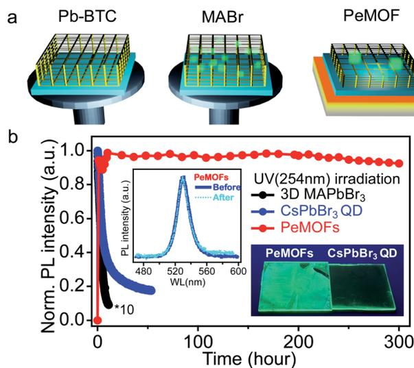
**Fig. 9** (a) Illustration of the PeMOF thin film fabrication process via a two-step spin coating method. (b) Time evolution of the normalized photoluminescence intensities of the 3D  $\text{MAPbBr}_3$  thin film,  $\text{CsPbBr}_3$  QD thin film and PeMOF thin film. The PL spectrum for a PeMOF thin film before and after UV irradiation is plotted in the inset, and a photo of the PeMOF versus QD thin films after aging is shown in the same plot. Reproduced from ref. 20 with permission.
