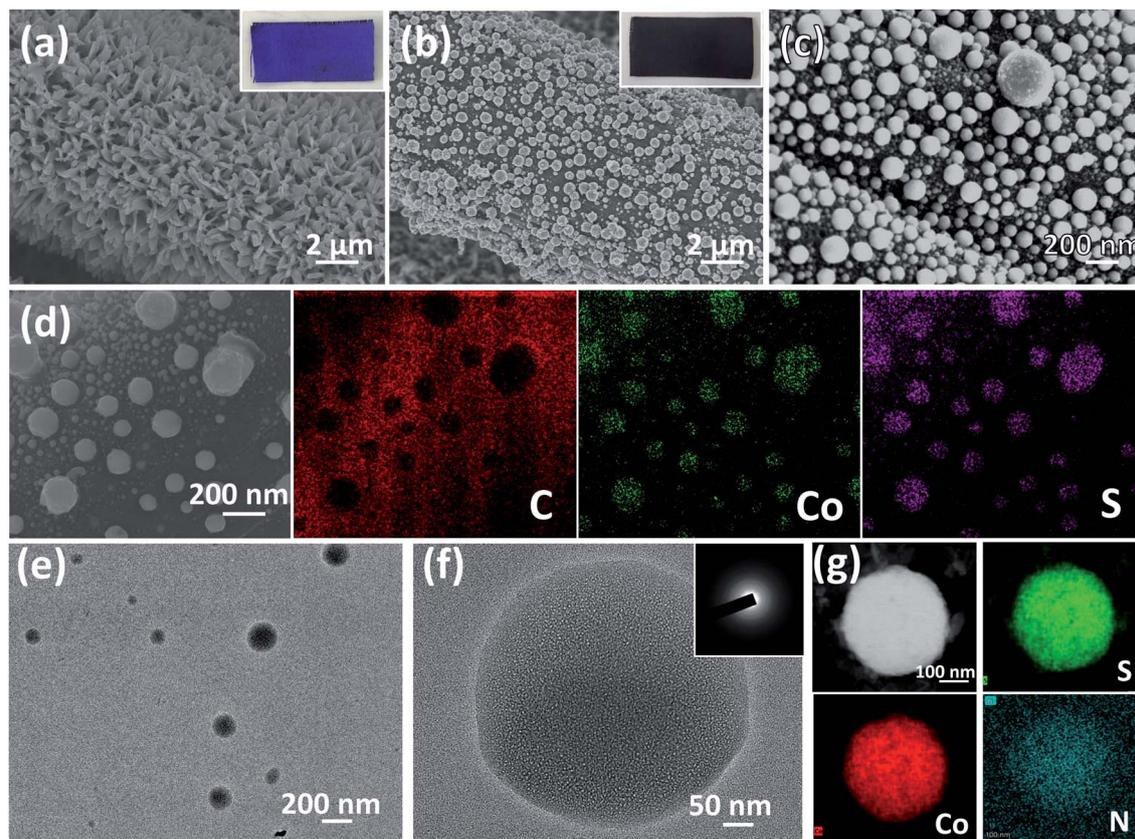
**Fig. 1** SEM images of Co-MOF/CC (a) and CoS<sub>x</sub>/CC-L (b and c). Insets are the corresponding photographs. (d) Corresponding EDS mapping of the C element, Co element and S element for CoS<sub>x</sub>/CC-L. TEM (e) and HRTEM (f) images of CoS<sub>x</sub>/CC-L. The inset in (f) is the SAED pattern of CoS<sub>x</sub>/CC-L. (g) Elemental mapping of CoS<sub>x</sub> nanospheres.
