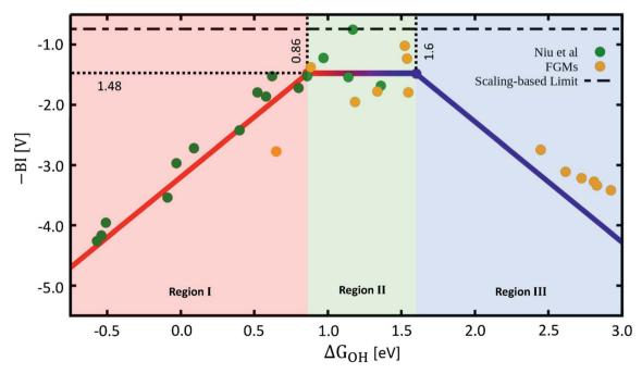
Fig. 2 Sabatier-type bifunctional volcano plot for OER/ORR electrocatalysis with the additive inverse of the bifunctional index (-BI) plotted as a function of  $\Delta G_{OH}$ . Datapoints labelled "Niu et al." and "FGMs" were taken from the respective publications. <sup>18,34,46</sup> Further details on the making of this plot appear in Sections S3-S6 in the ESI.†
