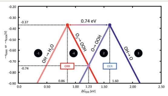
Fig. 1 Sabatier-type activity plots based on scaling relations for the OER (right) and ORR (left) as a function of  $\Delta G_{\text{OH}}$ . They are based on an energetic separation between \*OOH and \*OH of 3.20 eV, see Sections S1 and S2 in the ESI.† The most representative potential-limiting steps are noted in each case and have been determined statistically<sup>13,18</sup> from eqn (1)-(4) for the OER and the reverse equations for the ORR.
