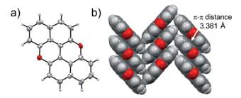
Fig. 7 Single-crystal X-ray structure of PXX. ORTEP representation (a) and (b) herringbone-type arrangement. Space groups:  $P2_1/c$ . Data taken from literature.<sup>52</sup> Atom colours: red O, grey C, white H.
