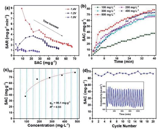
Fig. 7 (a) Ragone plots of SAC vs. SAR of HRBC-NTO/N-C-60 electrodes in different voltage with a flow rate of 25 mL min<sup>-1</sup>. (b) Desalination curves of HRBC-NTO/N-C-60 in different concentrations of NaCl solution at 1.4 V with a flow rate of 25 mL min<sup>-1</sup>. (c) Langmuir isotherm of HRBC-NTO/N-C-60. (d) Reusability of the desalination system in a 200 mg  $L^{-1}$  NaCl solution at 1.4 V with a flow rate of 25 mL min<sup>-1</sup>.
