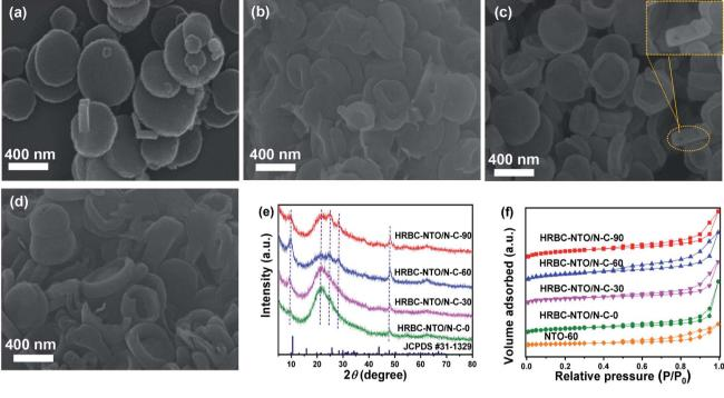
Fig. 3 SEM images of (a) HRBC-NTO/N-C-9. (b) HRBC-NTO/N-C-30, (c) HRBC-NTO/N-C-60, and (d) HRBC-NTO/N-C-90. (e) XRD patterns of HRBC-NTO/N-C-x. (f)  $N_2$  sorption isotherms of HRBC-NTO/N-C-x and NTO-60.
