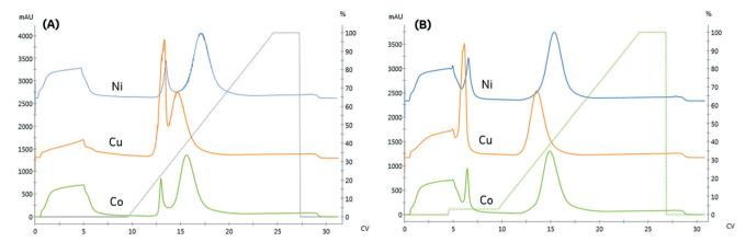
Fig. 2 Comparing the binding and elution profiles when the resin is charged with different divalent metals (nickel, copper, and cobalt). A fixed linear-gradient,  $\gamma = 11.3$ , was employed for trials where: (A) no imidazole is included in the sample or pre-elution wash (B) 15 mM imidazole is included in the pre-elution wash.
