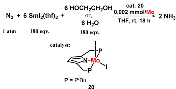
Fig. 24 NH<sub>3</sub> formation by molybdenum complex consisting of a PNP type anionic pyrrole ligand.
