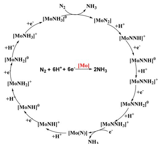
Fig. 5 Schrock–Yandulov cycle using complex 1 as a catalyst.
