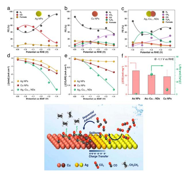
Fig. 10 (a–c) FEs for each gaseous product and for the main liquid product over (a) Ag NPs, (b) Cu NPs, and (c)  $Ag_1-Cu_{1.1}$  NDs. (d and e) Total current density (d) and partial current density for the electroreduction of  $CO_2$  (e) over Ag NPs, Cu NPs, and  $Ag_1-Cu_{1.1}$  NDs. (f) CO and  $C_2H_4$  mass activity of Ag NPs, Cu NPs and  $Ag_1-Cu_{1.1}$  NDs at -1.1 V vs. RHE. Reproduced with permission.<sup>114</sup> Copyright ©2018, American Chemical Society.
