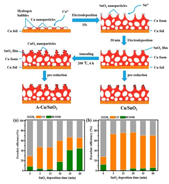
Fig. 5 (Up) Schematic drawing of the fabrication of  $Cu/SnO_2$  and  $A-Cu/SnO_2$ . (Bottom) Comparison of faradaic efficiencies of  $H_2$ , CO, and HCOOH for (a)  $Cu/SnO_2$  and (b)  $A-Cu/SnO_2$  electrodes with different deposition times at -1.0 V vs. RHE in  $CO_2$ -saturated 0.1 M KHCO<sub>3</sub>.<sup>73</sup>
