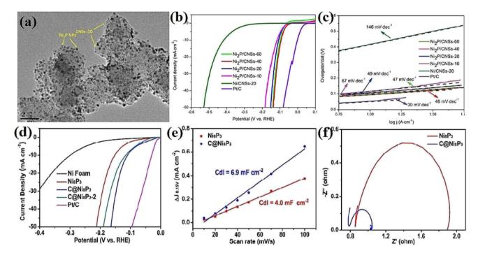
Fig. 14 Ni<sub>2</sub>P supported on carbon nanospheres: (a) TEM image, (b) LSV curves in 0.5 M  $H_2SO_4$  and (c) corresponding Tafel plots (reproduced from ref. 78 with permission from Elsevier, Copyright 2015). Carbon-coated Ni<sub>8</sub>P<sub>3</sub>: (d) LSV curves in 0.5 M  $H_2SO_4$ , (e) electrochemical double-layer capacitance and (f) EIS plots (reproduced from ref. 108 with permission from the America Chemistry Society, Copyright 2016).
