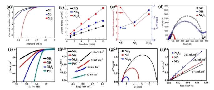
Fig. 8  $Ni_3S_2$ , NiS and NiS<sub>2</sub> electrocatalysts: (a) LSV curves in 1.0 M KOH, (b) electrochemical double-layer capacitance, (c) comparison of SSA (red) and ECSA (blue),<sup>49</sup> (d) EIS, (e) LSV curves in 1.0 M KOH, (f) corresponding Tafel plots, (g) EIS plots and (h) electrochemical double-layer capacitance.<sup>80</sup>
