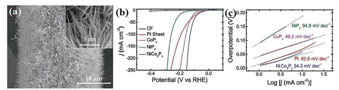
Fig. 12 NiCo<sub>2</sub> $P_x$  nanowire arrays: (a) SEM image, (b) LSV curves in 1.0 M KOH and (c) corresponding Tafel plots (reproduced from ref. 111 with permission from Wiley, Copyright 2017).
