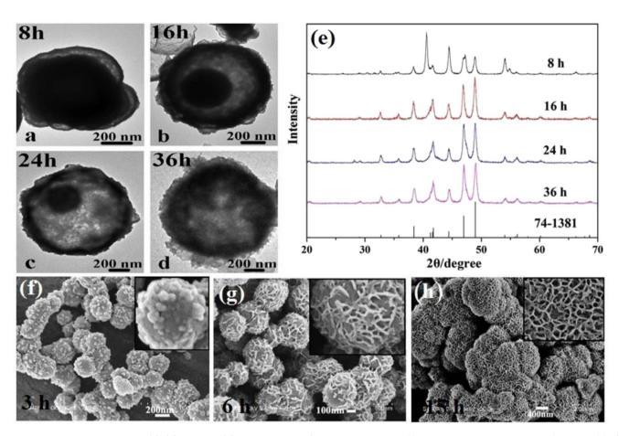
Fig. 3 Effect of synthesis time on: (a) – (d) structure, (e) crystalline phase (reproduced from ref. 60 with permission from Elsevier, Copyright 2015), and (f) – (h) morphology of nickel phosphides. 41
