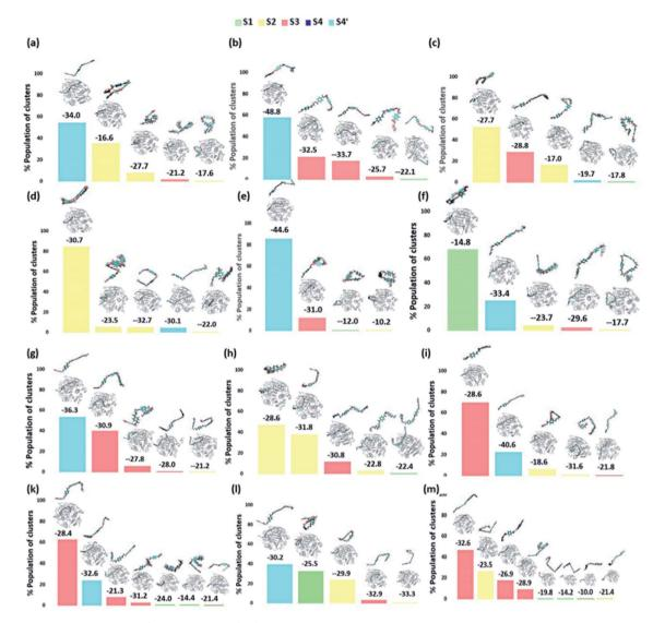
Fig. 6 The output of clustering on 12 different DM *TfCut2*-PET systems with the population percent of each cluster shown in *Y* axis. The average structure of each cluster along with its binding energy (kcal mol<sup>-1</sup>) obtained *via* MM-PBSA calculations is shown above the bar corresponding to each cluster. A zoomed image of PET is shown on top of each average structure.
