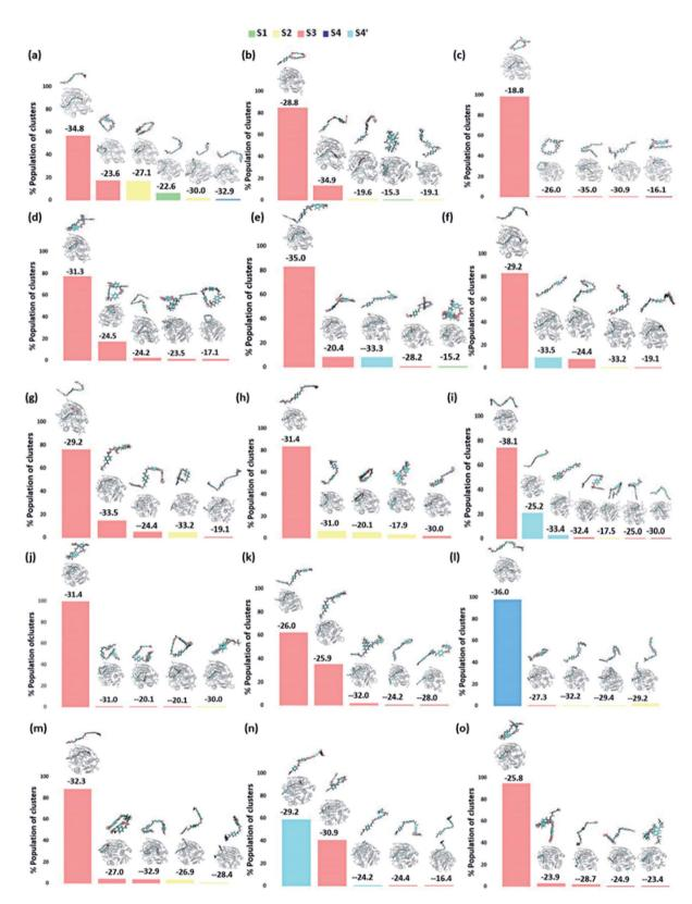
Fig. 5 The output of clustering on 15 different WT TfCut2-PET systems with the population percent of each cluster shown in Y axis. The average structure of each cluster along with its binding energy (kcal mol<sup>-1</sup>) obtained via MM-PBSA calculations is shown above the bar corresponding to each cluster. A zoomed image of PET is shown on top of each average structure.
