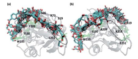
Fig. 2 Extended docked conformers of tetrameric PET in (a) 15 in WT TfCut2 (b) 51 in DM TfCut2. The region in the dotted circle indicates the terminal portion of the binding site.
