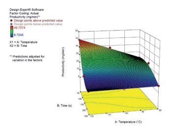
Fig. 7 Response surface for the productivity, in mg min<sup>-1</sup>, of DHMF from HMF.
