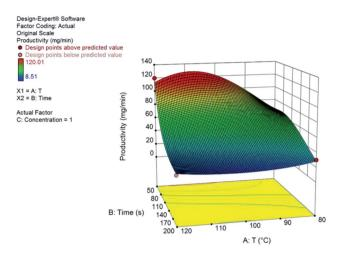
Fig. 3 Response surface for the productivity, in mg  $\min^{-1}$ , of furfuryl alcohol from furfural at 1.0 M. Coded variables are A for temperature and B for residence time.
