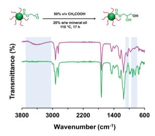
Fig. 7 FT-IR spectra recorded for PLMA $_{63}$ -PGlyMA $_{89}$  prior to (green spectrum) and after reacting with 50% v/v aqueous acetic acid at 110 °C for 17 h (pink spectrum). In principle, this simply involves acid-catalyzed epoxy ring-opening with water but in practice side-reactions also occur, which leads to extensive core-crosslinking of the nanoparticles.
