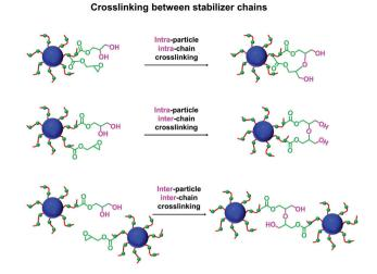
Scheme 3 Schematic representation of the various reactions that can occur when reacting  $P(LMA_{50}-stat-GlyMA_9)-PMMA_{67}$  nanoparticles with trace water by heating a 20% w/w copolymer dispersion in mineral oil to 110 °C. Following the initial epoxy ring-opening reaction, the resulting hydroxyl groups can react with the remaining epoxy groups. This leads to both intra-particle and/or inter-particle crosslinking.
