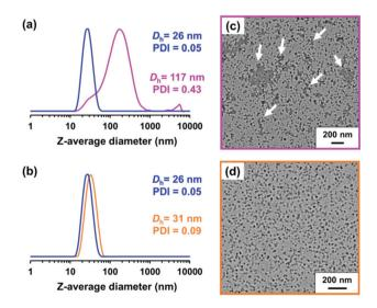
Fig. 6 DLS particle size distributions recorded for P(LMA $_{50}$ -stat-GlyMA $_{9}$ )-PMMA $_{67}$  nanoparticles both prior to heating (blue trace) and after heating to 110 °C for 40 h at (a) 20% w/w solids (pink trace) or (b) 1.0% w/w solids (orange trace). Corresponding TEM images obtained for (c) the 20% w/w dispersion and (d) the 1.0% w/w dispersion after heating to 110 °C for 40 h.
