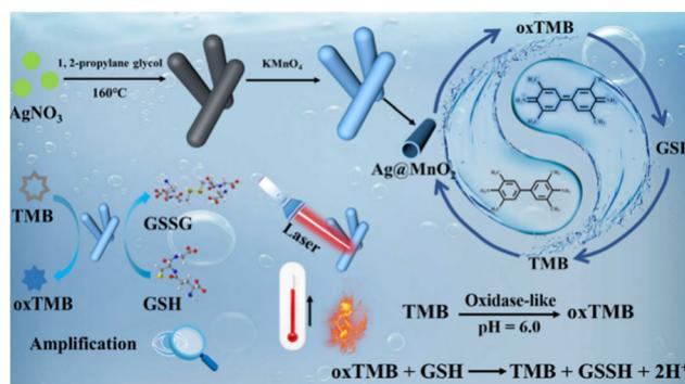
**Scheme 1** Schematic illustration of the synthesis of Ag@MnO<sub>2</sub> nanowires and the process of dual-mode colorimetric and photothermal detection for GSH.
