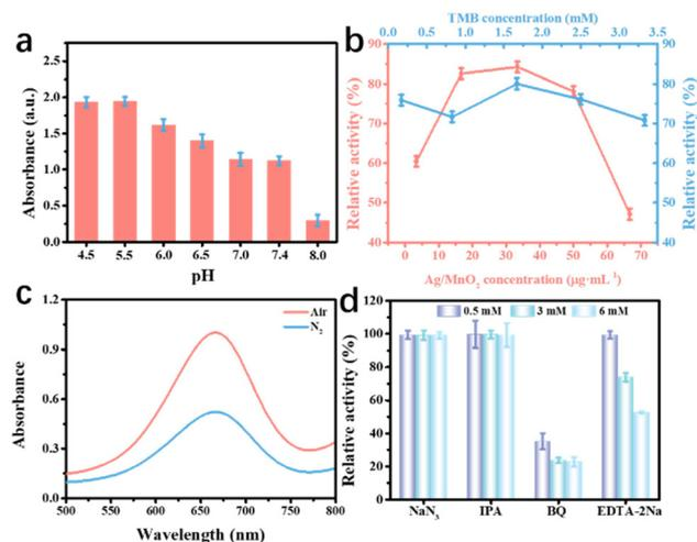
**Fig. 4** Experimental condition optimization and mechanism study. The oxidase-like activity of Ag@MnO<sub>2</sub> depended on: (a) pH and (b) concentration; (c) effect of dissolved oxygen; (d) the relative activity of the Ag@MnO<sub>2</sub> catalytic system with ROS scavengers.
