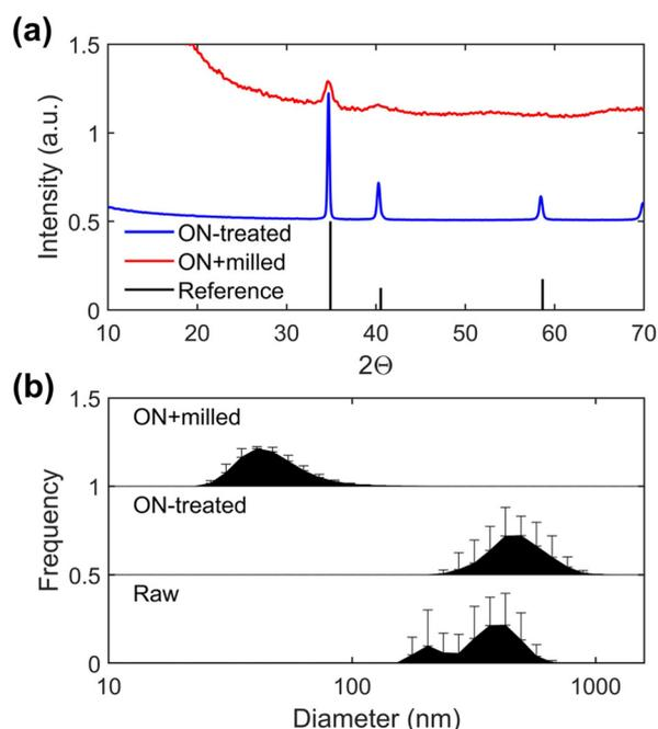
Fig. 1 Production of TiH<sub>2</sub> nanoparticle dispersion. (a) pXRD of powder following octylamine treatment and subsequent wet ball milling, with TiH<sub>2</sub> reference (PDF 00-025-0982). (b) DLS size distributions following octylamine treatment and subsequent ball wet ball milling.
