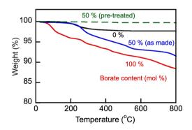
Fig. 2 TGA heating ramp (10 °C min $^{-1}$ ) of as-made carbonate (Li $_{1.24}$ K $_{0.76}$ CO $_3$ ), borate (Li $_{1.5}$ Na $_{1.5}$ BO $_3$ ) and as-made and pre-treated blend (1:1 mol/mol, sample no. 3 in Table 1) in nitrogen atmosphere. The blend sample was pre-treated by its equilibration at 600 °C in N $_2$  atmosphere for 1 h. Numbers stand for nominal initial content of borate (mol $_3$ ) in the samples.
