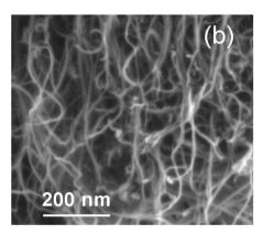
Fig. 14 TEM (a) and SEM (b) microphotographs of MWCNT found in the products of  $CO_2$  electrolysis conducted in borate ( $Li_{1.5}Na_{1.5}BO_3$ ) and eutectic carbonate ( $Li_{1.24}K_{0.76}CO_3$ ) blend (1:1 mol/mol) at 550 °C.
