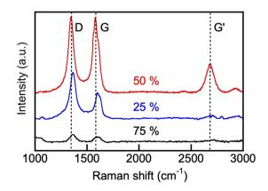
**Fig. 15** Raman spectra of the products of  $CO_2$  electrolysis conducted in borate ( $Li_{1.5}Na_{1.5}BO_3$ ) and eutectic carbonate ( $Li_{1.24}K_{0.76}CO_3$ ) blends at 550 °C. Numbers indicate the initial borate concentration in the blend (mol%). For other detail, see Experimental.
