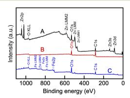
Fig. 10 XPS spectra of the original galvanized steel electrode (A), the same electrode utilized in the CO2 electrolysis at 550 °C in molten Li, K borate/Li, Na carbonate (1:1 mol/mol) blend (B), and the same electrode after cleaning its surface of the CNT deposited during the electrolysis (C). For electrolysis conditions, see Experimental.
