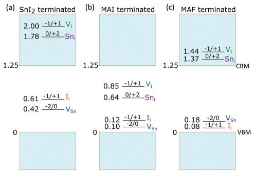
Fig. 4 Lowest thermodynamic charge transition levels of point defects on the  $Snl_2$ , MAI and MAF(001) terminated MASnl<sub>3</sub> surfaces. All energies are referred to the valence band maximum (VBM) of the respective surface model. The notation q/q' used in the figure refers to charge transition levels (q/q') as defined in Computational details.
