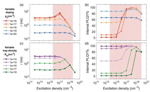
Fig. 1 Simulated carrier lifetime (a and c) and internal PLQY (b and d) as solutions to the system of equations eqn (1)-(5). (a and b) With variable doping density and trap density fixed at 1016 cm<sup>-3</sup> (parameters listed in Table S1 (ESI†)); (c and d) with variable trap density and doping density fixed at 1018 cm<sup>-1</sup> (parameters listed in Table S2 (ESI†)). Shaded regions indicate the experimental measurement ranges showed in Fig. 2 and 3
