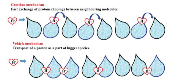
Fig. 6 Proton transport mechanism in the fuel cell
