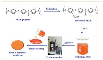
Fig. 5 Schematic preparation of SPEEK membranes.
