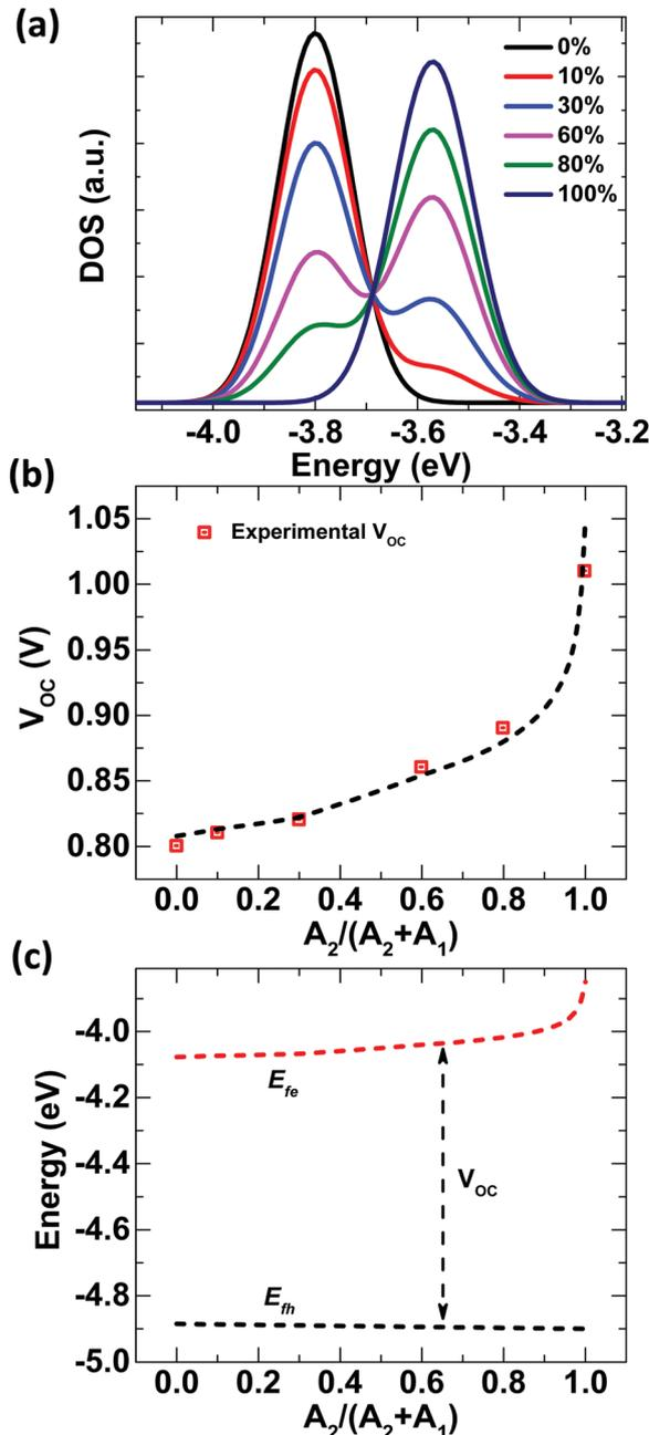
Fig. 3 Changes in DOSs for different A<sub>1</sub>:A<sub>2</sub> concentrations plotted against energy using eqn (2) and eqn (3); (b) experimental  $V_{\text{OC}}$  values (red squares) fitted with a population occupancy DOS model (dashed line); and (c) QFL splitting for different A<sub>1</sub>:A<sub>2</sub> ratios in D ternary blend solar cells, obtained from population occupancy in a Gaussian disorder model.
