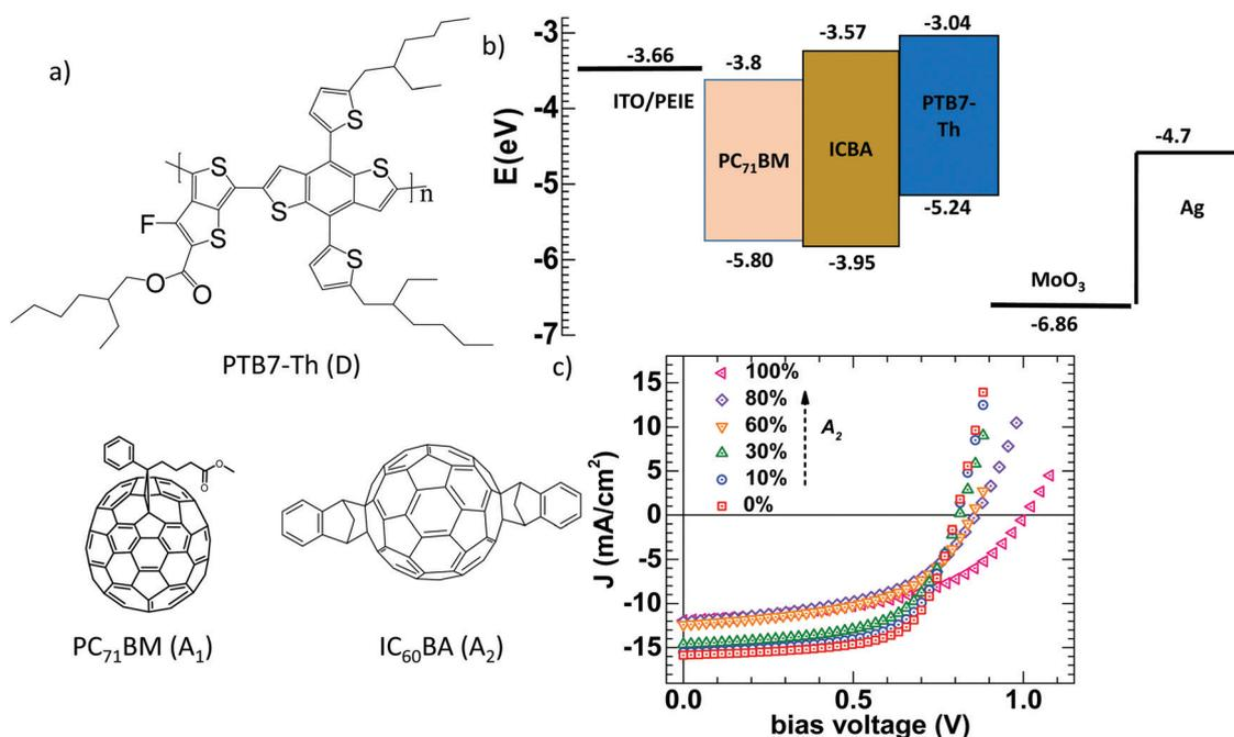
Fig. 1 (a) The molecular structures of D, A<sub>1</sub>, and A<sub>2</sub>; (b) the device structure with the HOMO and LUMO energy levels (A<sub>1</sub> and A<sub>2</sub>,<sup>35</sup> D<sup>33</sup>) and work functions of various layers; and (c) illuminated  $J$ - $V$  characteristics for different A<sub>1</sub>:A<sub>2</sub> ratios in D polymer based solar cells under AM1.5 illumination.
