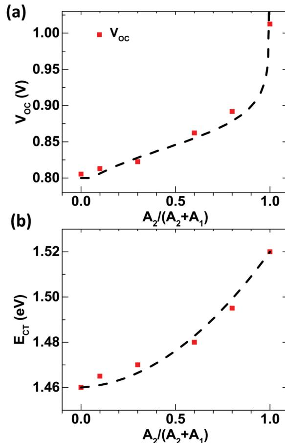
Fig. 2 Alloy composition vs. (a) changes in V<sub>OC</sub> using the double-diode model (the dotted line represents the fitting of experimental V<sub>OC</sub> values with eqn (2)) and (b) changes in the E<sub>CT</sub> value of the BHJ alloy composition determined from sensitive EQE studies (the dotted line represents the fitting of experimental E<sub>CT</sub> values with eqn (3)).
