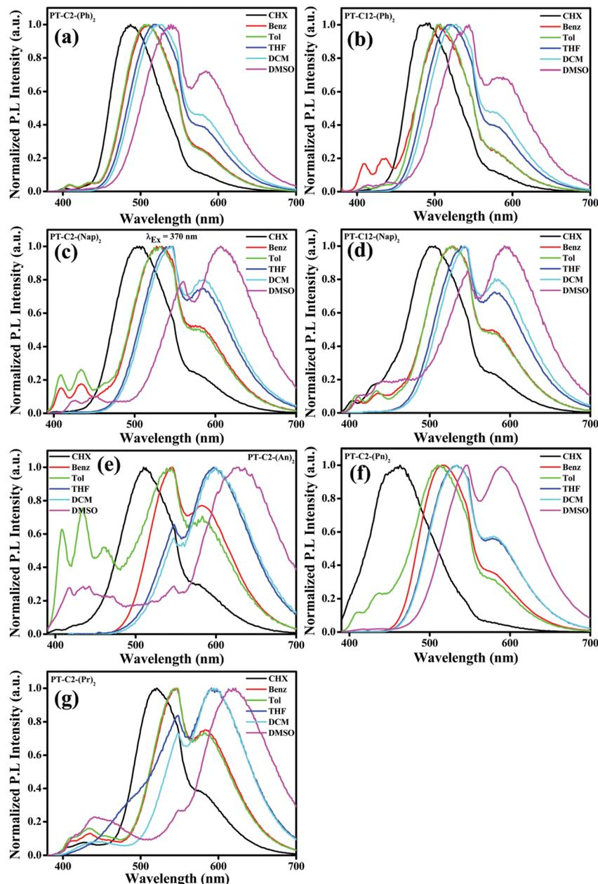
Fig. 2 Emission spectra of (a) PT-C2-(Ph)<sub>2</sub>, (b) PT-C12-(Ph)<sub>2</sub>, (c) PT-C2-(Nap)<sub>2</sub>, (d) PT-C12-(Nap)<sub>2</sub>, (e) PT-C2-(An)<sub>2</sub> and (f) PT-C2-(Pn)<sub>2</sub> and (g) PT-C2-(Pr)<sub>2</sub> in solvents (cyclohexane (CHX), benzene (Benz), toluene (Tol), DCM, THF and DMSO) of varying polarities ( $\lambda_{\text{Ex}} = 370$  nm).
