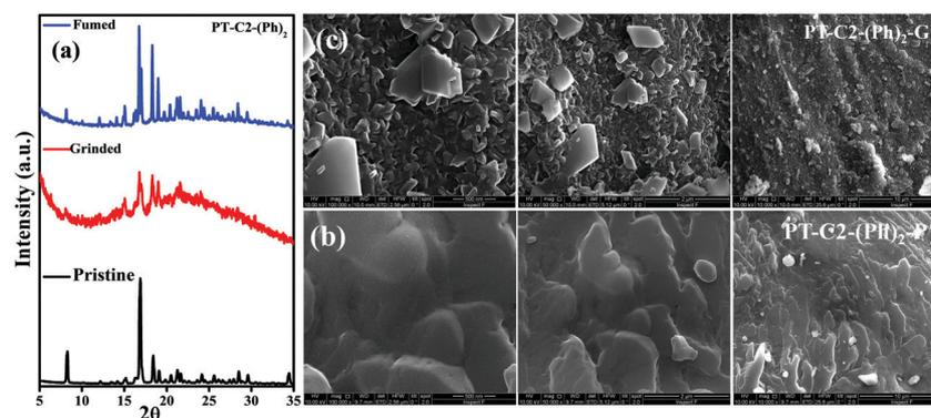
Fig. 7 (a) P-XRD patterns of the pristine, ground, and fumed samples of PT-C2-(Ph)<sub>2</sub>, SEM images of PT-C2-(Ph)<sub>2</sub> in its (b) pristine (PT-C2-(Ph)<sub>2</sub>-P) and (c) ground (PT-C2-(Ph)<sub>2</sub>-G) states.
