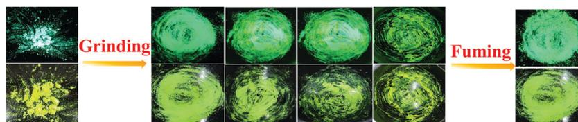
Fig. 5 Images of PT-C2-(Ph)<sub>2</sub> solids in different states (pristine (left), ground/fumed (right)) under 365 nm light and normal light.
