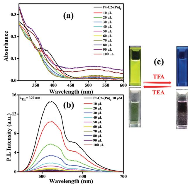
Fig. 8 Absorption (a) and emission spectra of (b) PT-C2-(Pn)<sub>2</sub> in CHCl<sub>3</sub> (conc. 10<sup>-5</sup> M) on titration with known amounts of TFA (10–100 μL). (c) Emission photographs of PT-C2-(Pn)<sub>2</sub> in reversible response to TFA and TEA under UV light (top) and normal light (bottom).
