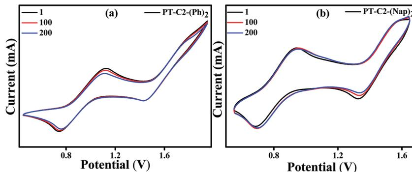
Fig. 4 Cyclic voltammograms ( $200 \text{ mV s}^{-1}$ ) of PT-C2-(Ph)<sub>2</sub> (a) and PT-C2-(Nap)<sub>2</sub> (b) (1st, 100th and 200th cycles) in DCM (ca. 1.0 mM) recorded in CH<sub>2</sub>Cl<sub>2</sub> using TBAPF<sub>6</sub> (0.1 M) as the supporting electrolyte.
