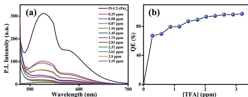
Fig. 9 Emission spectra of the (a) PT-C2-(Pn)<sub>2</sub> film on titration with known amounts of TFA. (b) Concentration versus quenching efficiency [QE (%)] under increased TFA vapor concentration.
