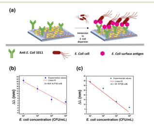
Fig. 7 Schematic of the mechanism of capturing *E. coli* cells promoted by the Ab incorporated on the plasmonic substrate. (a) Optical shift  $(\Delta\lambda)$  as a function of *E. coli* concentration in the incubation dispersion, reported on a logarithmic scale for *E. coli* recognition experiments in the presence of SYTO  $9^{\text{TM}}$  (b) and in the absence of SYTO  $9^{\text{TM}}$  (c).
