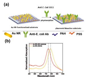
Fig. 5 Schematic of the procedure for bioactivating Au NR 800functionalized substrates with the captured antibody able to recognize F coli cells (a) Spectroscopic characterization of the bioactive plasmonic substrate after the incorporation of the Ab (yellow track) shows an optical red-shift of 40 nm with respect to the Au NR 800functionalized substrate (b).
